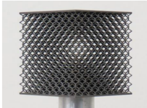
Figure 3: Rhombic dodecahedral lattice structure made of 316SS using SLM. Photo courtesy of LLNL.
