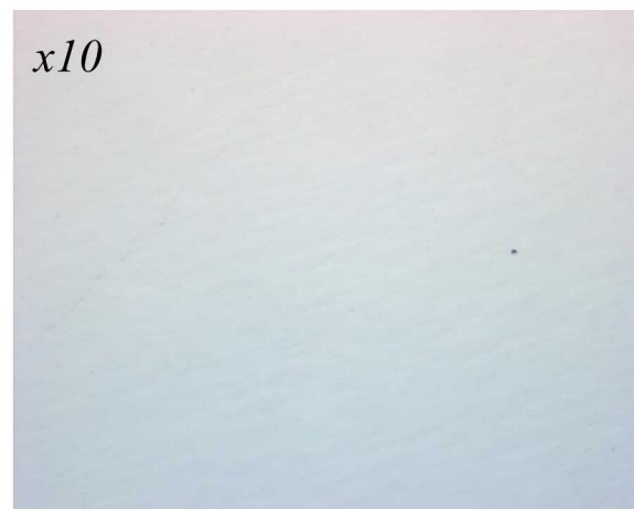
GaN after 10 min. KOH etching at 70 °C
