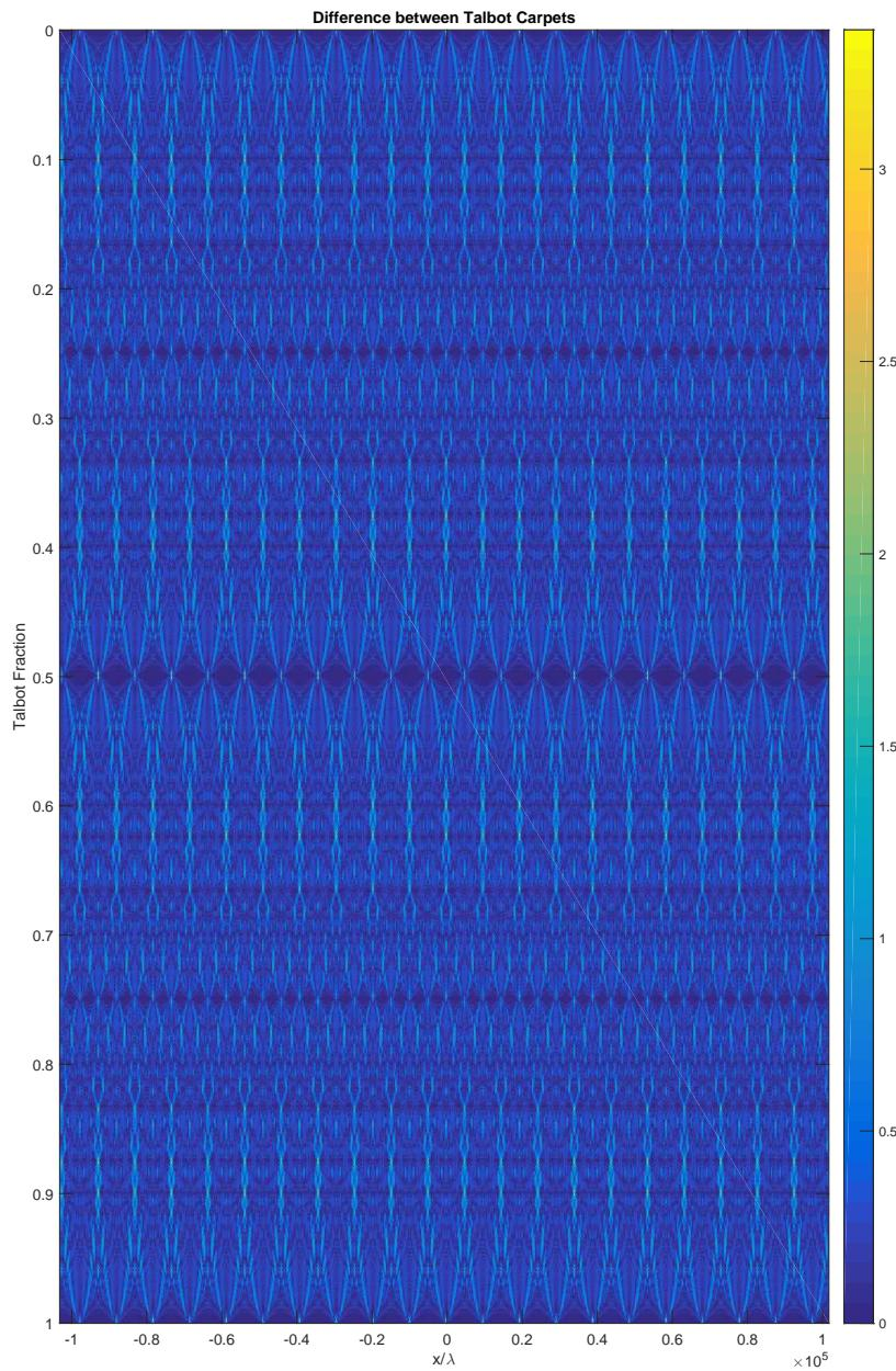
Figure 1. Difference in output Talbot carpet for slightly differing input gratings
