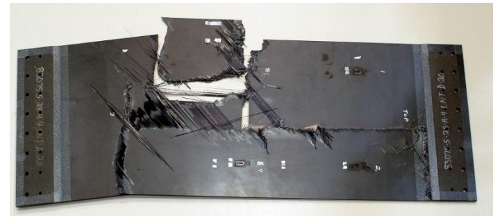
Typical crack growth in a notched laminate (photo courtesy Boeing)
