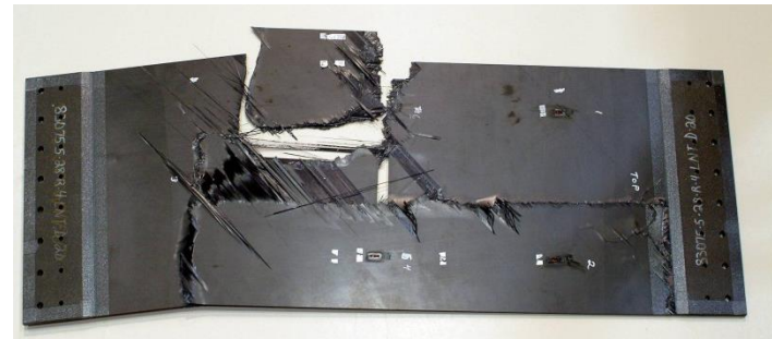
Typical crack growth in a notched laminate (photo courtesy Boeing)
