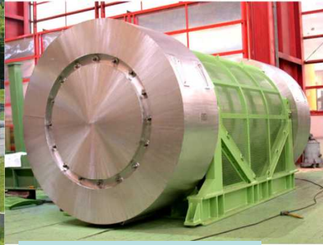
NAC-STC rail cask Courtesy Yankee Rowe
