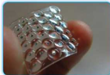
Figure 1 – Sample of Microscale Solar PV Cells Embedded in Silicone (Courtesy: Sandia National Laboratories)
