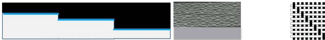
Figure 1: Specimens are constructed of carbon fiber reinforced plastic (CFRP) [4 ply [0/90]_2 ], 8 ply [0/90]_4 ], and 12 ply [0/90]_6 ], preimpregnated 8 harness-satin weave with UF3352 TCR™ Resin
