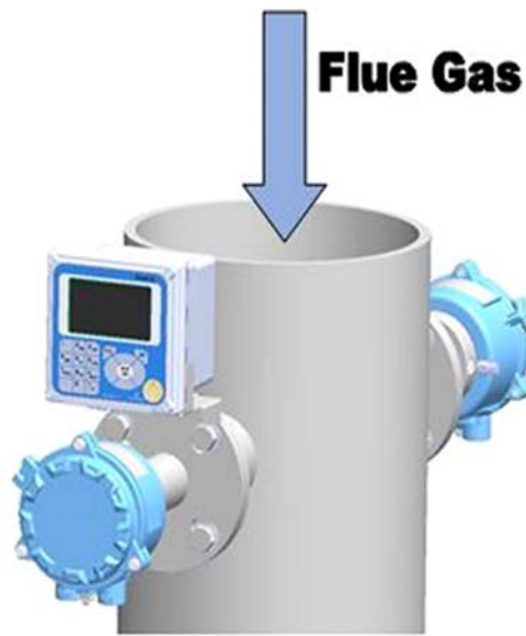
Fig. 19. A typical installation of TDL analyzer across the gas pipe or combustion duct.
