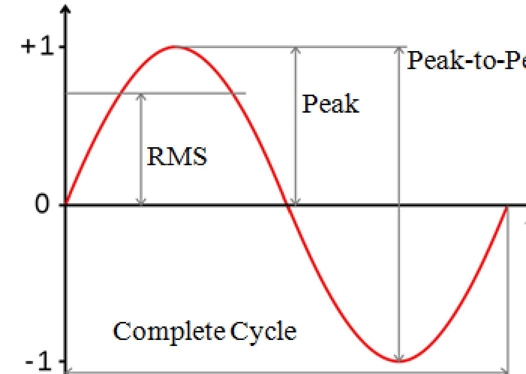
Selecting a signal to represent the largest signal amplitude may be subject to interpretation. Generally, the signal will have an amplitude equal to the clip level of the sensor. We have chosen to define the largest signal as the RMS value of a full-scale sinusoid. The advantages of using the RMS of a sinusoid are:
