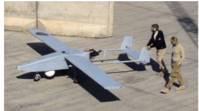
Copperhead miniSAR mounted on a Tiger Shark UAV
