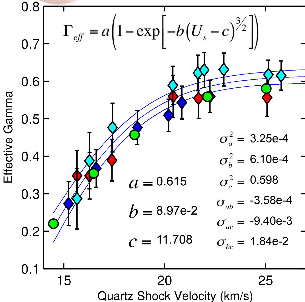
The similar trend in  $\Gamma_{eff}$  for all three release standards suggests that the Mie-Grüneisen, constant  $\Gamma_{eff}$  model with linear  $U_s - u_p$  Hugoniot reference adequately describes the release path to quite low pressure states
