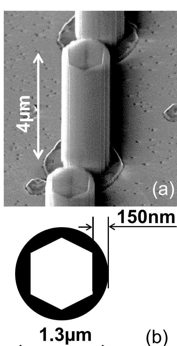
(a) The SEM image and (b) scheme of the cross-section of the as fabricated GaN nanotube laser. CCD images of the GaN nanotube laser excited (c) below and (b) above lasing threshold
