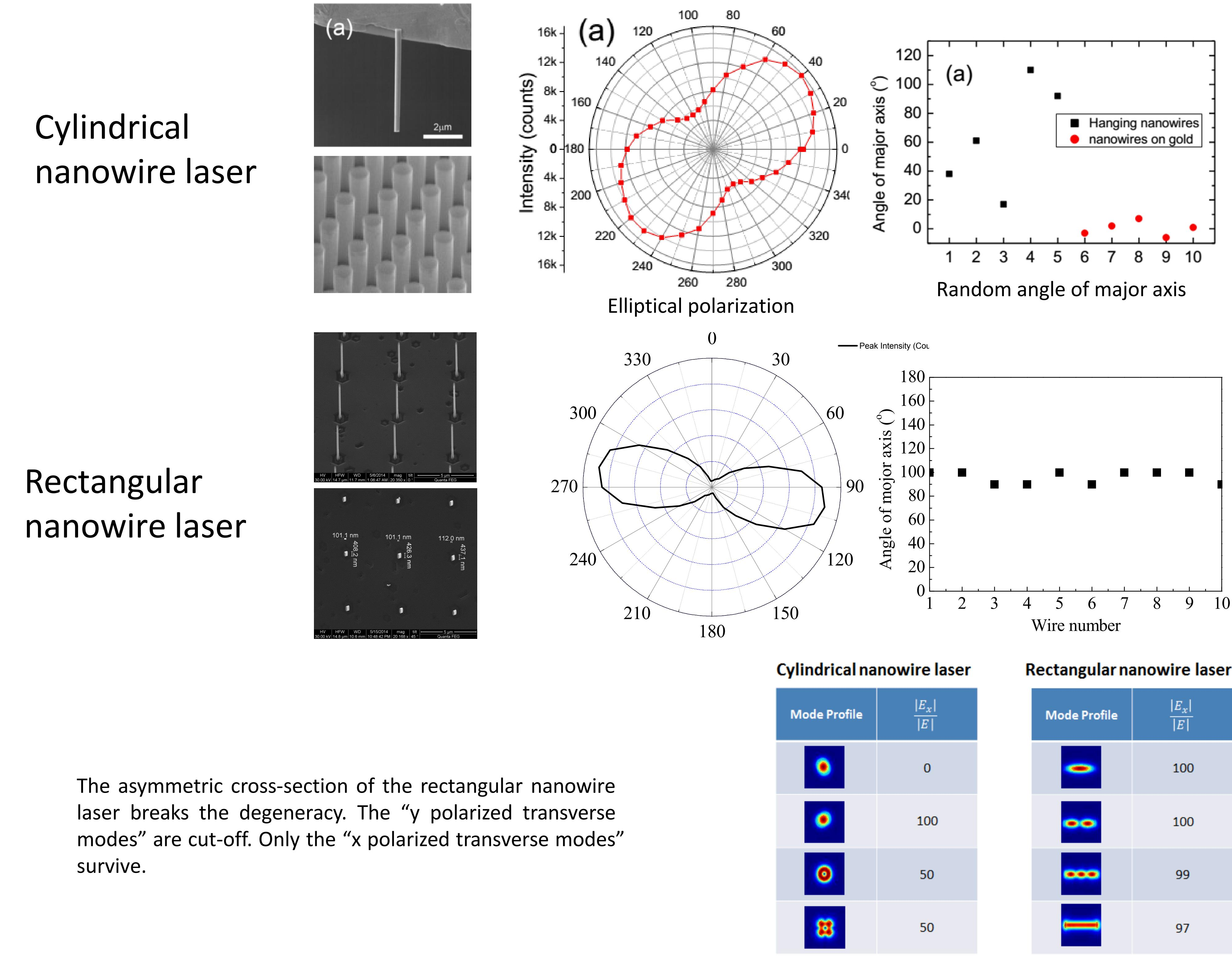
The asymmetric cross-section of the rectangular nanowire laser breaks the degeneracy. The "y polarized transverse modes" are cut-off. Only the "x polarized transverse modes" survive.
