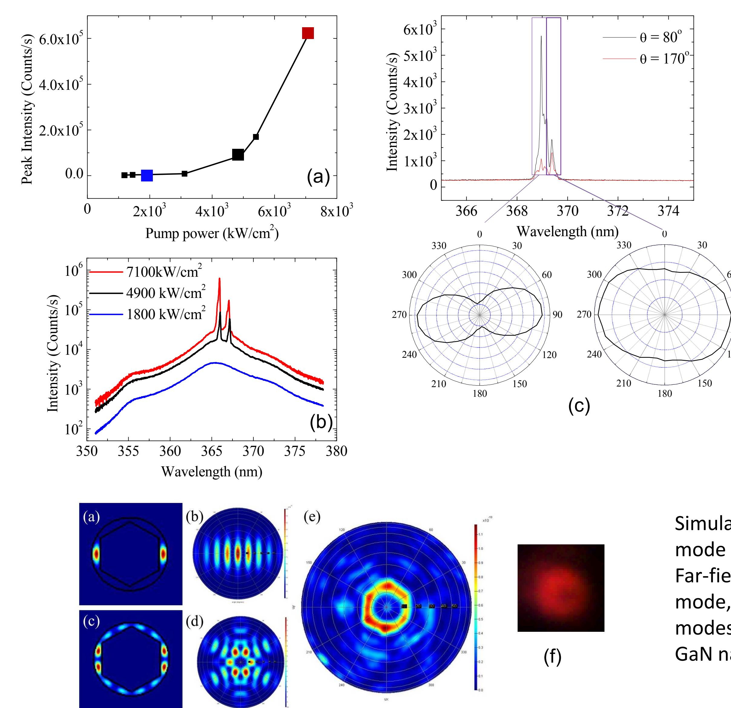
(a) Light-light curve and (b) spectra of the GaN nanotube laser. when the GaN nanotube is excited over a pump power density of approximately 4500 kW/cm<sup>2</sup>, the peak intensity increases with a much larger slope as the pump power density increases, implying that stimulate emission dominates and the nanotube is excited above lasing threshold.
