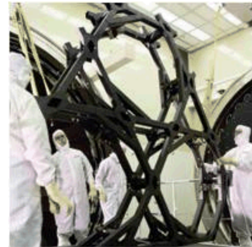
James Webb Space Telescope carbon fiber backplane (Hexcel)
