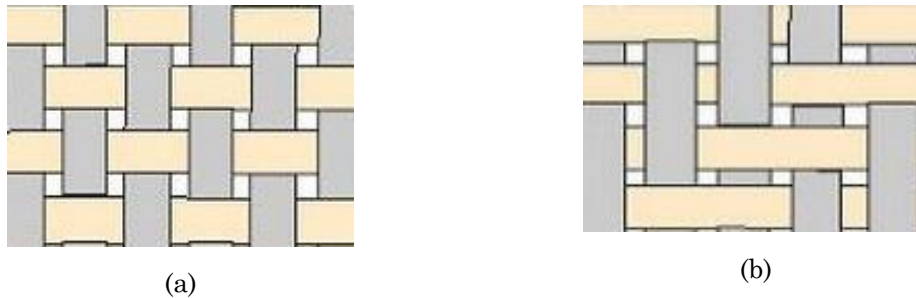
Figure 3.1-13. Illustration of (a) 1x1 plain weave and (b) 2x2 twill weave.
