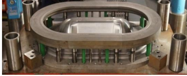
Figure 3.2-85. Geometry of the double-dome punch and the binder.
