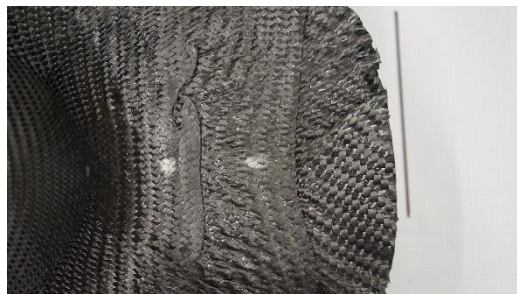
Figure 3.2-92. Folding of the prepreg after low temperature preforming especially at the edge.
