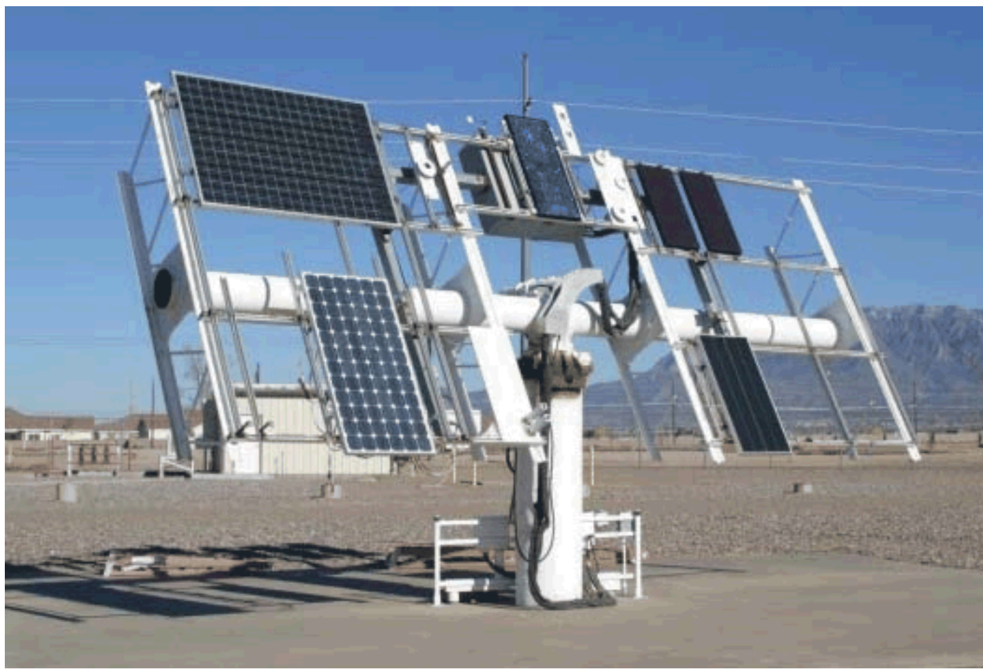
Two axis trackers are used to minimize AOI throughout the day. POA irradiance can be used directly in performance models.
