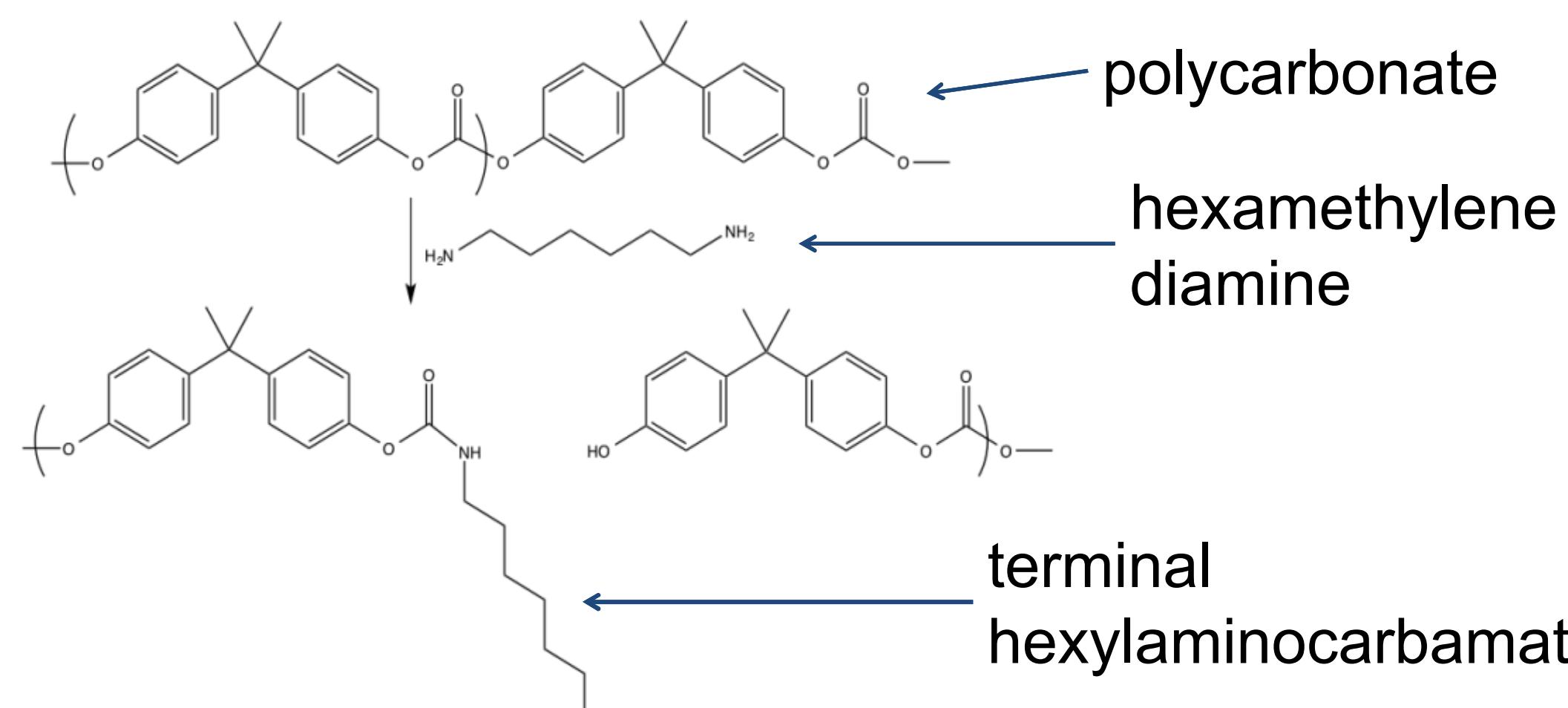
Upon addition of the aqueous hexamethylene diamine solution to the PC surface, the carbonyl group undergoes nucleophilic addition by the diamine. This reaction results in scission of the polymer chain and the formation of a terminal hexylaminocarbamate.
