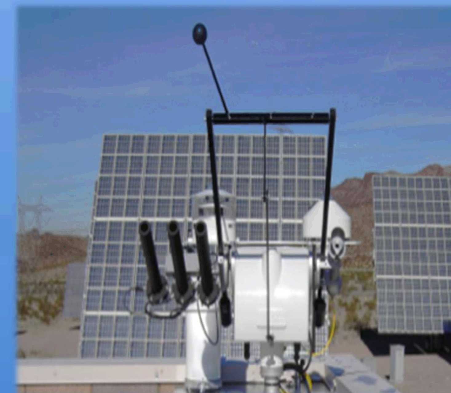
Figure 6. Solar tracker measures direct normal irradiance at the Nevada RTC, with 84kW CPV system in the background.
