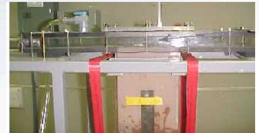
erosion measurement flume
