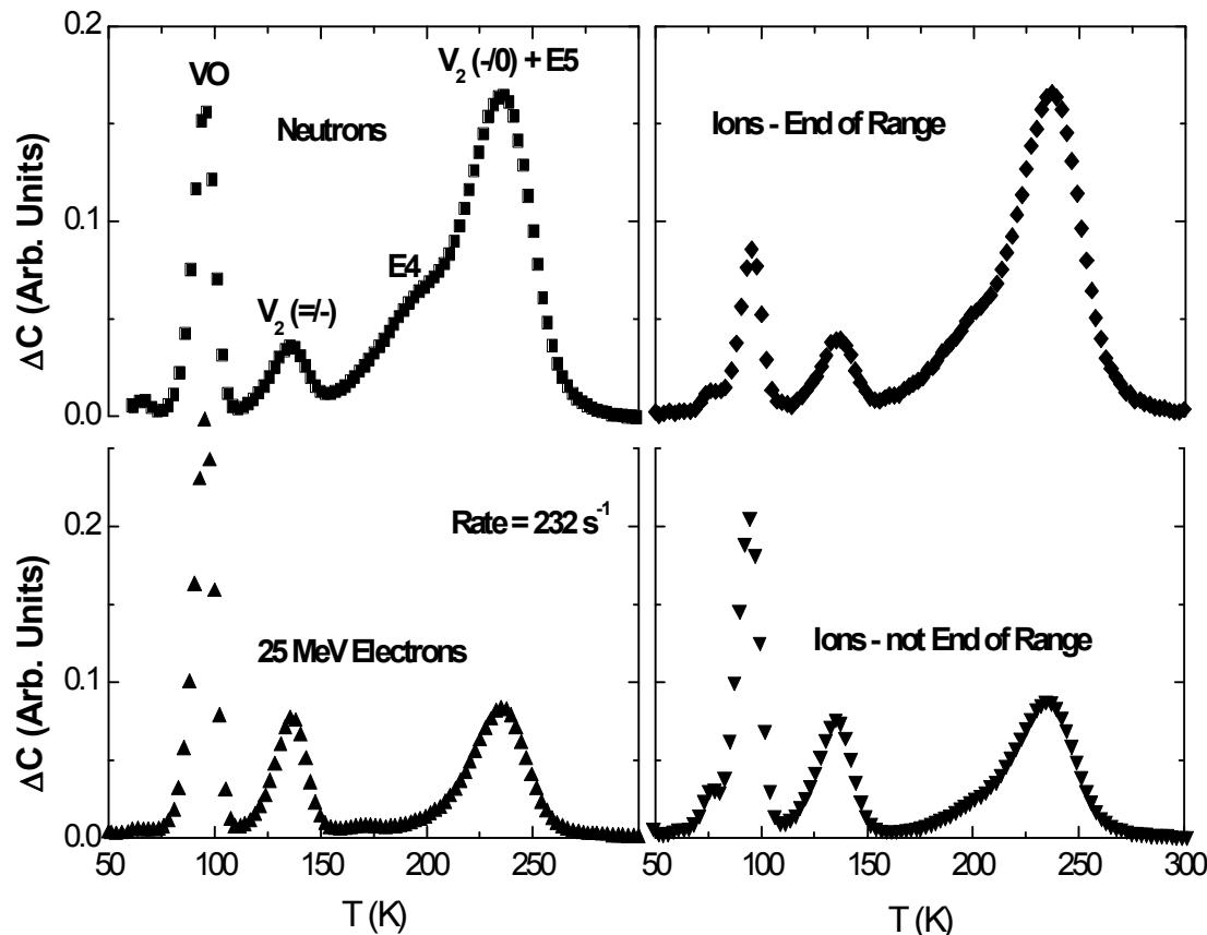
Uniquely identify and count the type and number of fundamental defects caused by irradiation
