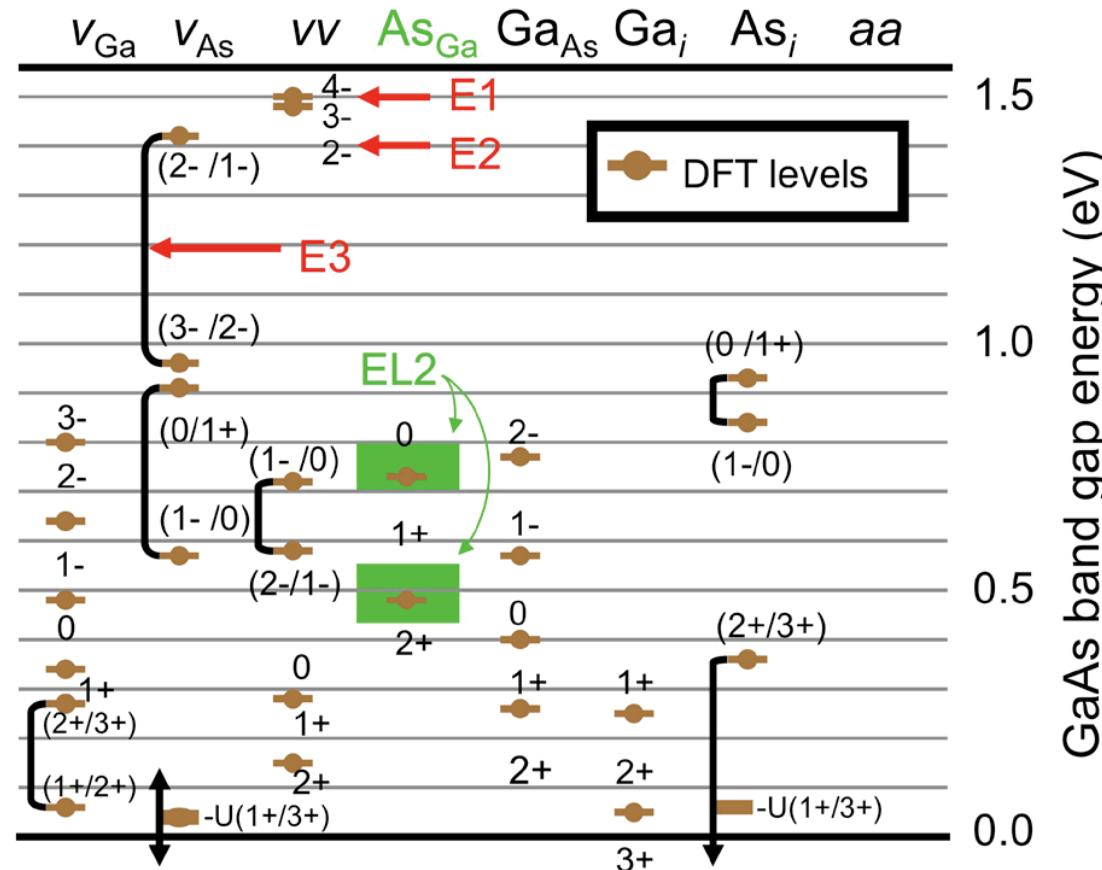
Pure prediction: a GaAs radiation defects Rosetta Stone
