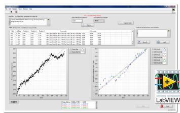
SNL technologists have also created and developed an interactive LabVIEW data analytics interface that receives RoboMET.3D generated data files and plots removal rate, slice number and laser measurement data all in real-time as the data is collected during the experiment. This provides opportunity to adjust the experiment in-situ should anomalies occur during sectioning.
