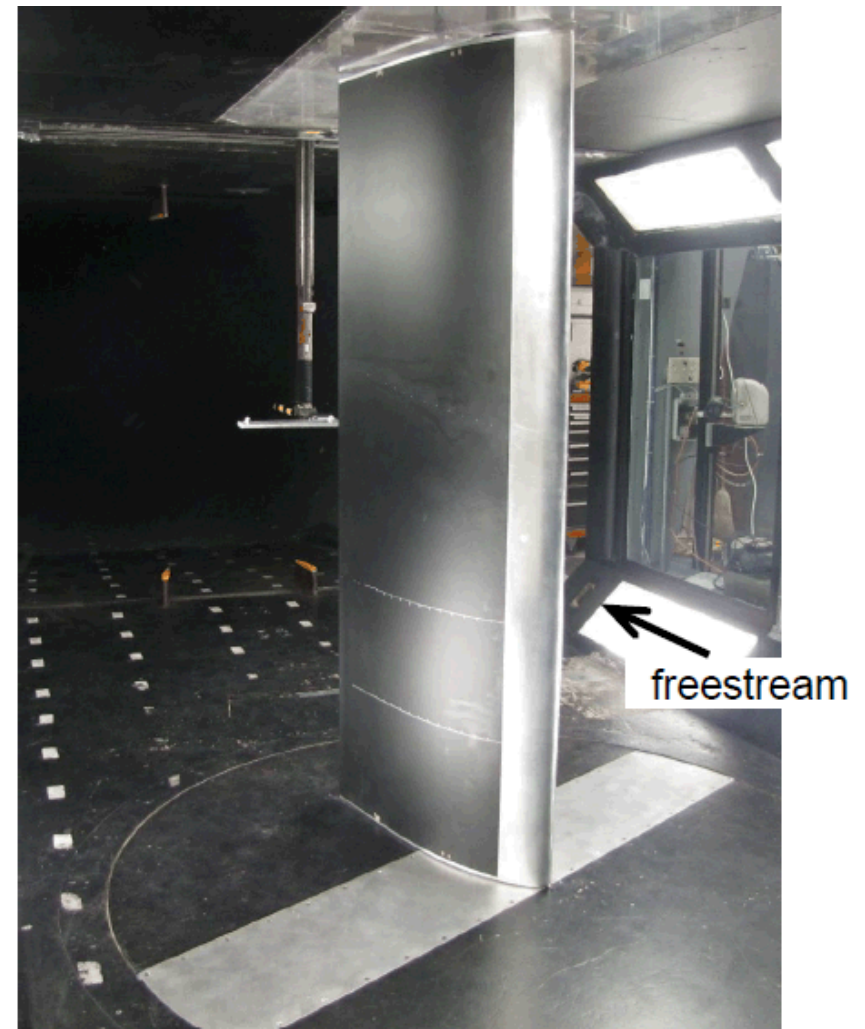
Model installed in wind tunnel
