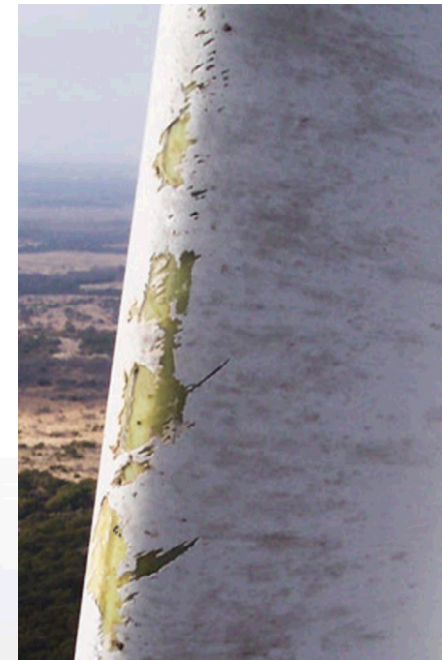
Leading edge blade erosion 4
