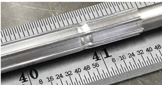
Fig. 6. Collapsed finned tube with visible dummy pellet recess.
