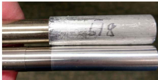
Fig. 2. Bimetallic transition joints – as-received condition (top) and joint with aluminum flashing removed (bottom).
