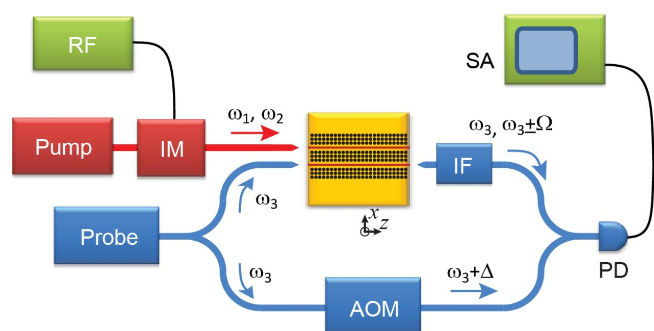
Pump: pump laser at 1547 nm
