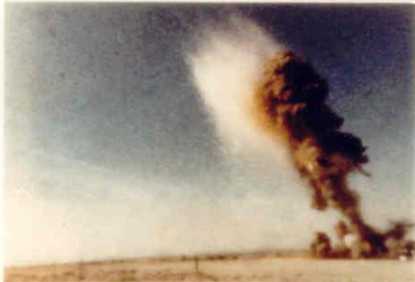
t = 1.0 \text{ sec.} EJECTED MELT REACHES MAXIMUM HEIGHT. PARTICLES BEGIN SEPARATION FROM AEROSOL.
