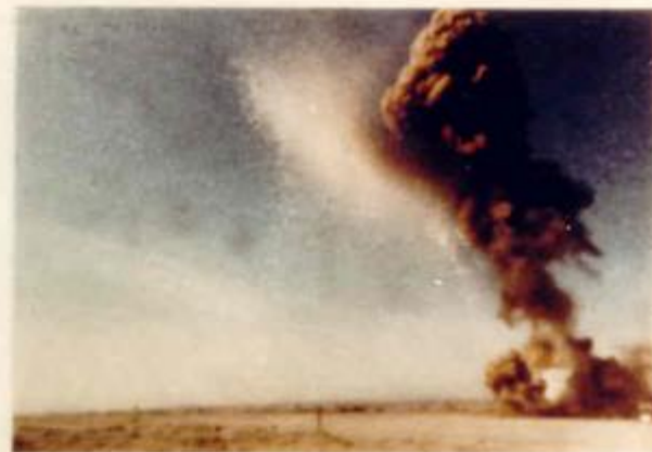
t = 1.5 \text{ sec.} SEPARATION COMPLETE. PARTICLES FOLLOWING PARABOLIC TRAJECTORIES.
