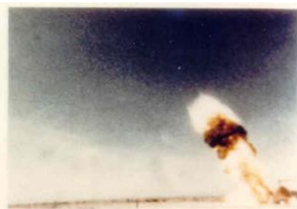
t = 0.5 \text{ sec.} MELT EJECTION FROM CAVITY COMPLETE. AEROSOL CLOUD BEGINS TO FORM.
