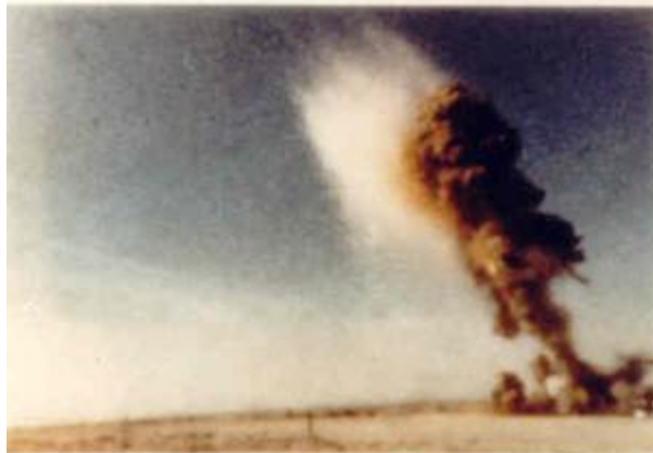
t = 1.0 \text{ sec.} EJECTED MELT REACHES MAXIMUM HEIGHT. PARTICLES BEGIN SEPARATION FROM AEROSOL.
