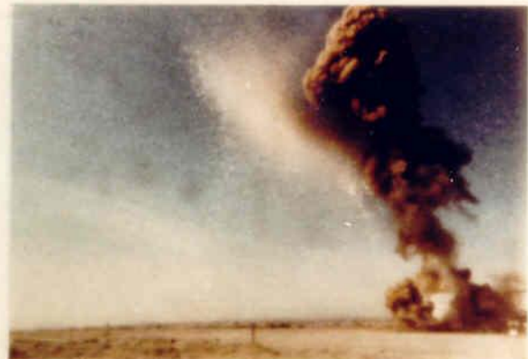
t = 1.5 \text{ sec.} SEPARATION COMPLETE. PARTICLES FOLLOWING PARABOLIC TRAJECTORIES.
