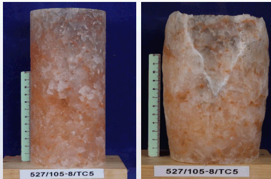
Room Temperature Triaxial Test Sample of WIPP Salt at 3.0 MPa Confining Stress
