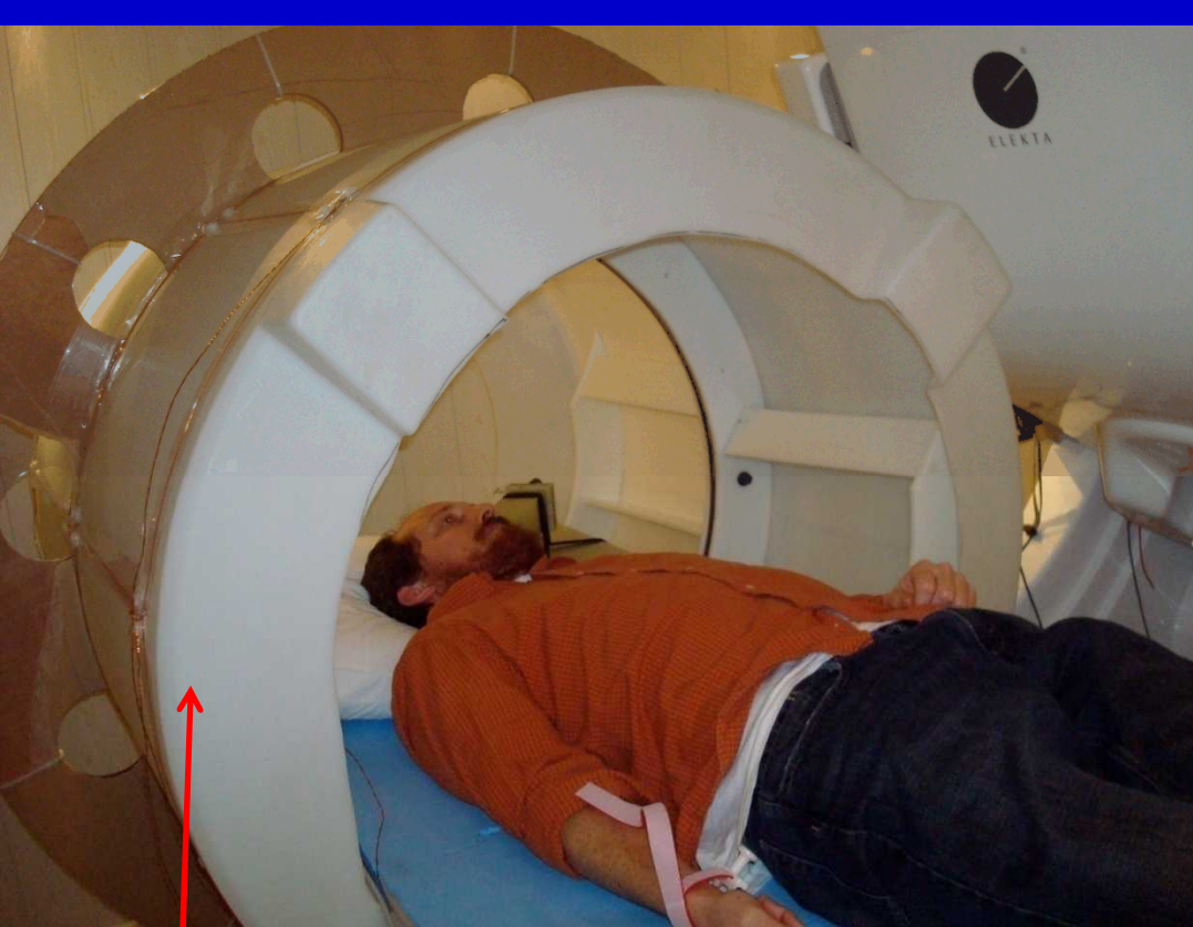
18-coil field cancellation system for reducing the field from \sim 100 nT to < 1 nT
