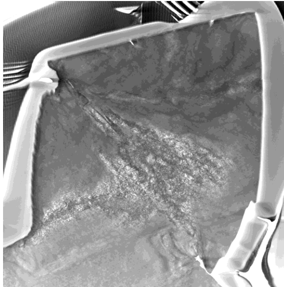
TEM image of FIB cross section of tested pillar
