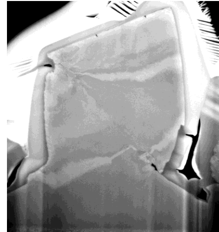
SEM image of FIB cross section of tested pillar
