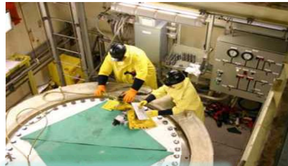
Lid Installation of a TN-32 Cask
