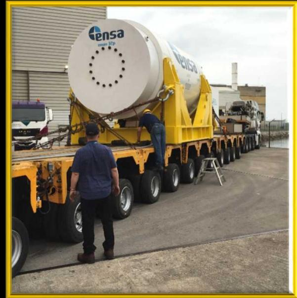
***Loading on 16-axle, 110 foot-long heavy-haul truck.
