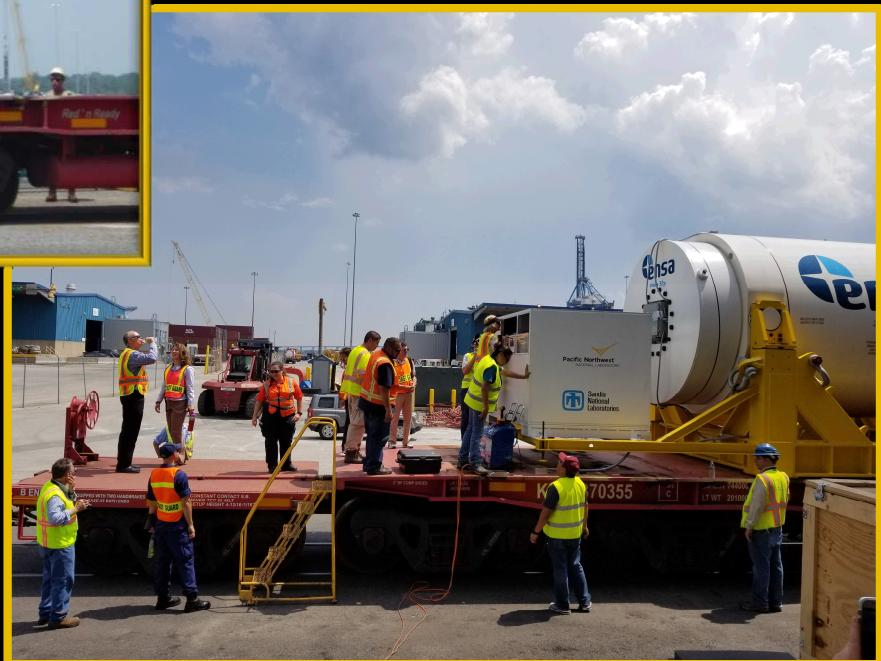
*While not a 2043 railcar, the 12-axle Kasgro railcar is expected to bound the strains and accelerations seen in a 2043.*
