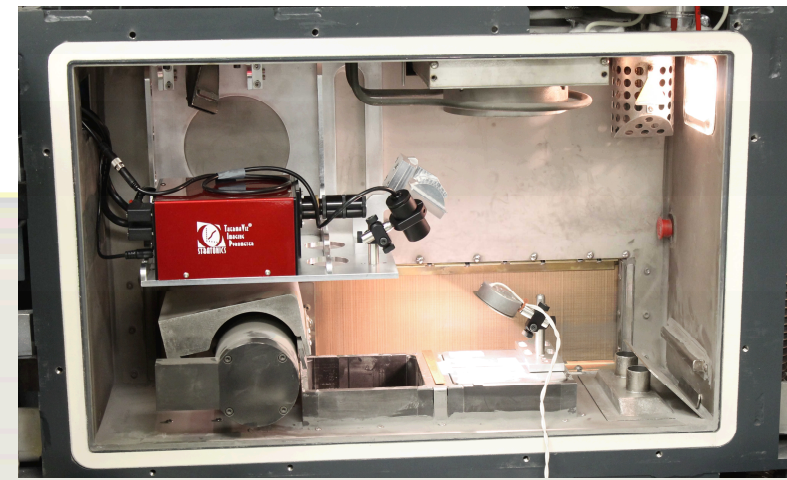
ThermaViz installed in the 3D Systems ProX 200
