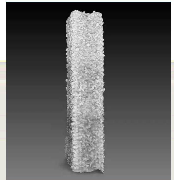
captured defect holes part CT image, Zeiss Xradia 520 Versa, voxel resolution ~ 2 \mu\text{m} , Harlan Brown-Shaklee
