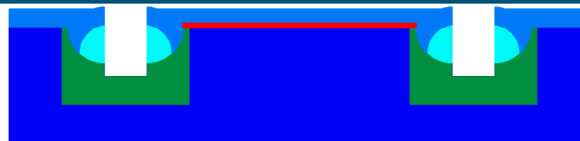
2. Vias are etched through Si Cap, remaining oxide, and into the implanted region
