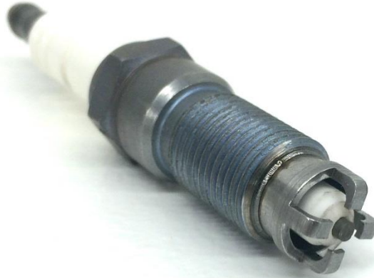
Figure 7 - Modified spark plug. The base plug is a Brisk spark plug, the four-pronged tip was laser welded onto the shell to create four 1.5mm gaps.
