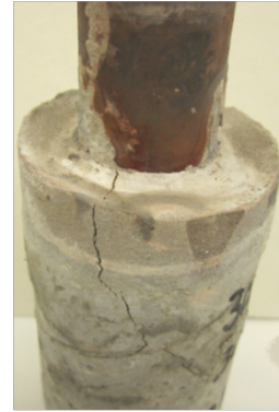
Cracks developed in MGF-modified TSRC by high sheath shear bond strength
