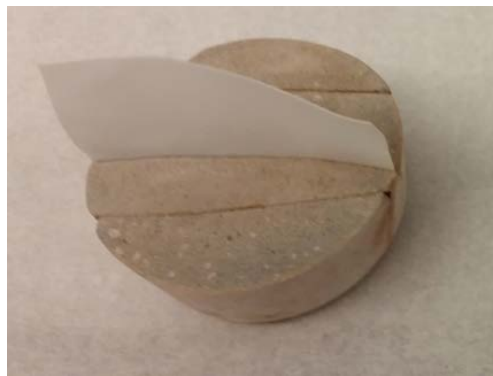
Figure 27. Cement sample with a Teflon sheet of 0.5 mm thickness to create a well-defined artificial crack of 0.5 mm wide and about 2 mm deep.
