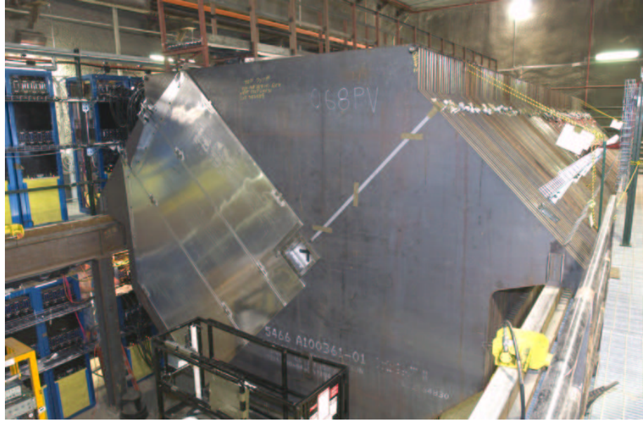
Figure 3.10: The Near detector on July 9, 2004. At the time the photo was taken the detector was still being installed. The leading plane is partially instrumented and in the Hadron Calorimeter section of the detector [39].
