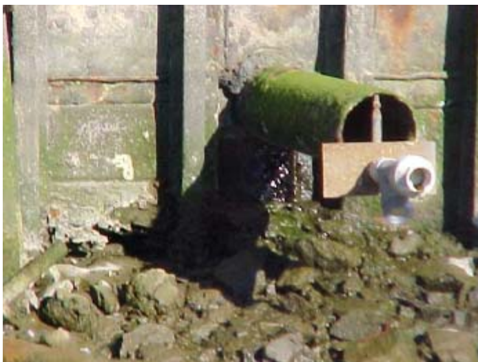
Clockwise from upper left: Y-trap prepared in laboratory, Y-trap deployed in municipal outfall at head of Lauritzen Channel, Y-trap deployed in 8-in. pipe in northeast Lauritzen Channel, collecting sediment from strainer removed from Y-trap from 8-in. pipe.
