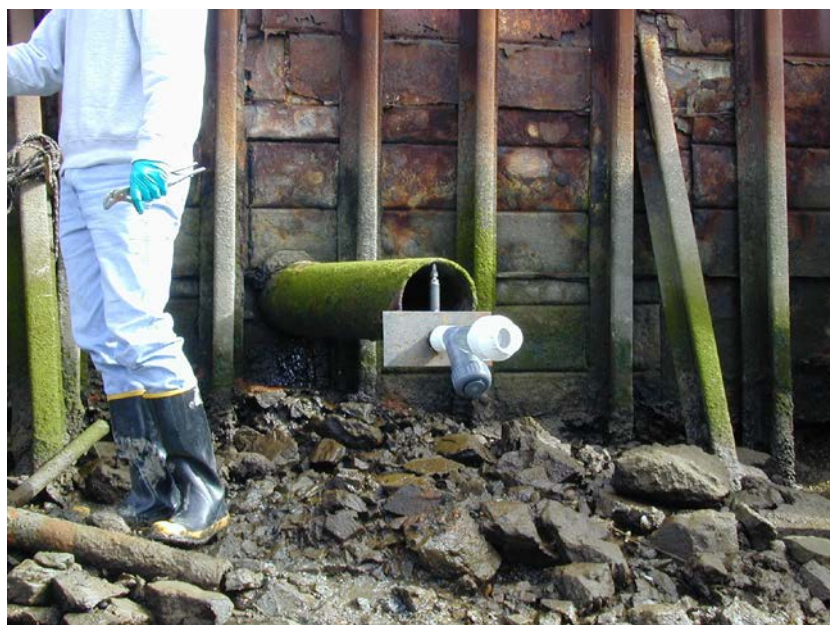
Photo 2 - Sediment Trap 2 (ST-2) and Passive Sampler 2 (PS-2) installation. 2/6/02.
