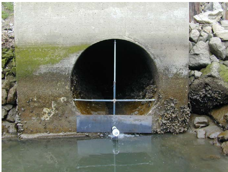
Photo 1 - Sediment Trap 1 (ST-1) and Passive Sampler 1 (PS-1) installation. 2/6/02.
