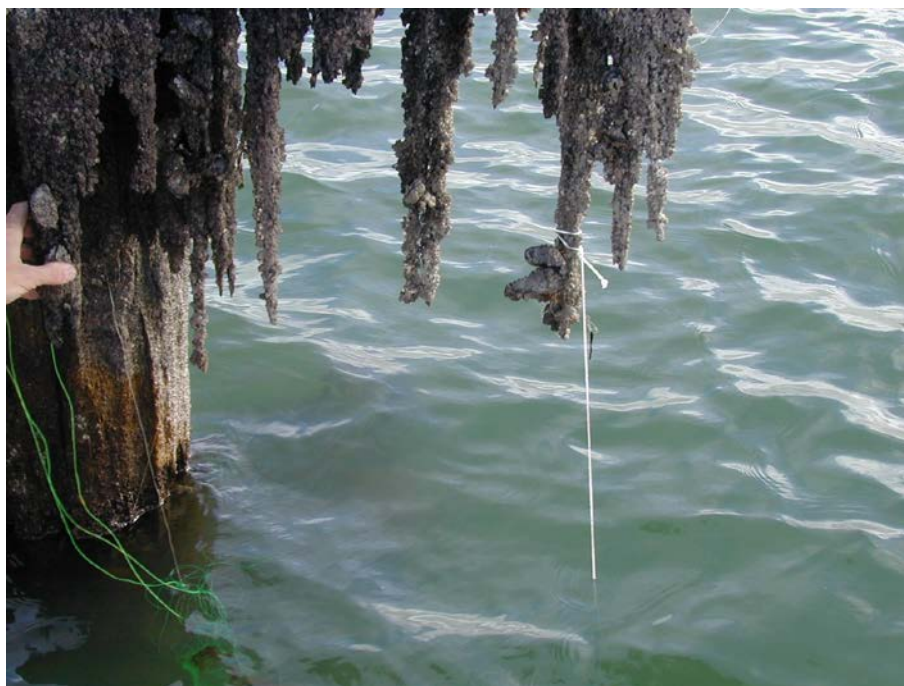
Photo 6 - Passive Sampler 8 (PS-8) installation, Richmond Inner Harbor Channel. 2/6/02.
