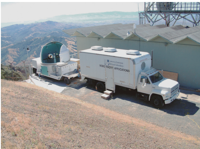
The portable transceiver system of the Secure Air–Optic Transport and Routing Network (SATRN) in position on Mt. Diablo. One of the longest high-capacity terrestrial links ever achieved, SATRN established a 28.2-km laser-communications link from Mount Diablo to LLNL at a single-channel data rate of 2.488 Gbit/s. This is equivalent to ~1600 conventional T1 data lines, 400 TV channels, or 40,000 simultaneous phone calls.
