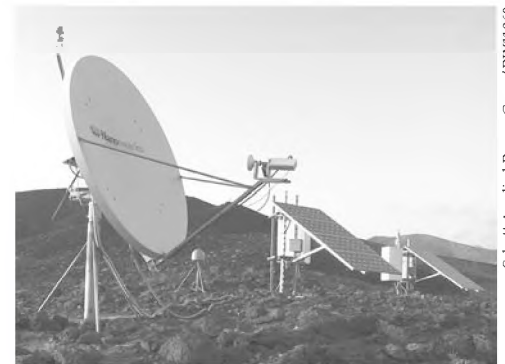
This earthquake-monitoring system operates on solar power.
