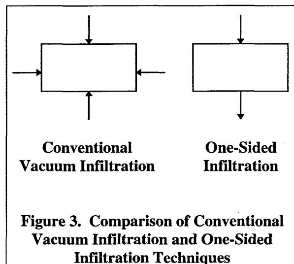
**Figure 3. Comparison of Conventional Vacuum Infiltration and One-Sided Infiltration Techniques**
