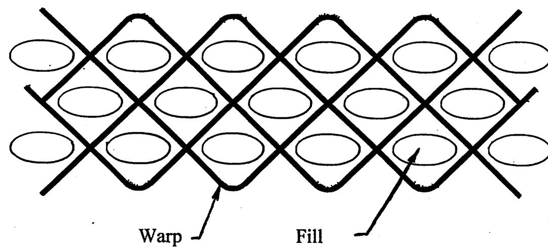
**Figure 1. Schematic of multi-layer fabric where the warp yarns provide axial and radial reinforcement while fill yarns provide hoop reinforcement.**
