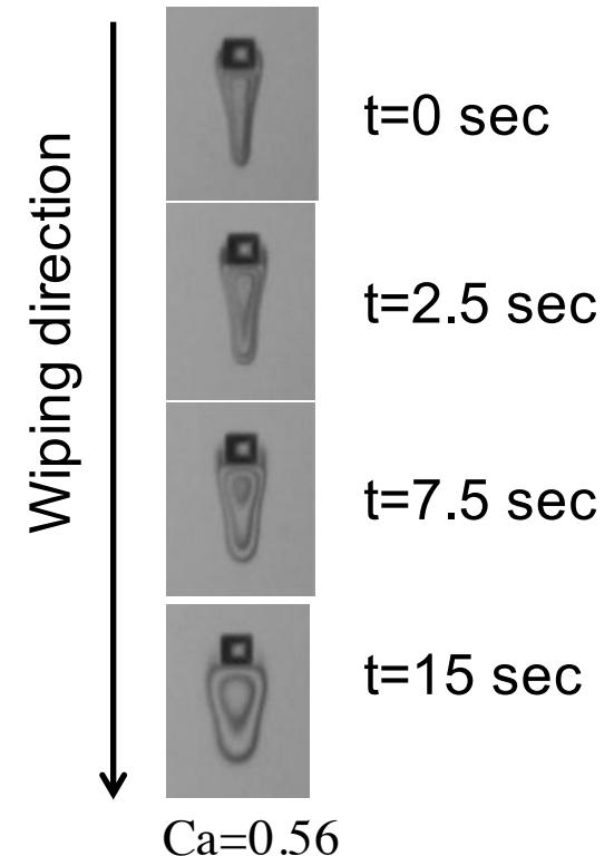
Dragout is currently one of the largest challenges for gravure patterning precise mesoscale features (OTFTs, OLEDs, sensors)
