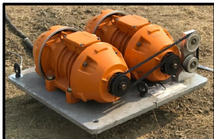
MicroVib™ Seismic Source atop Mounting Plate
