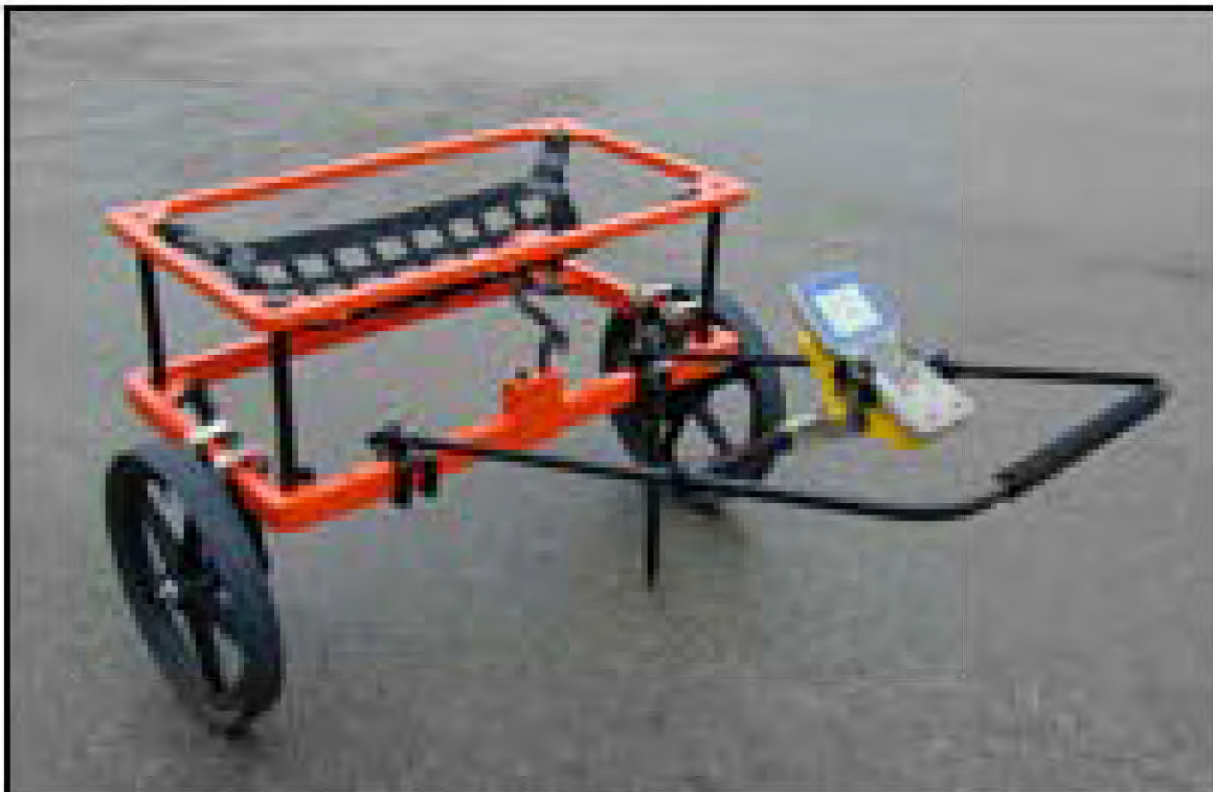
Figure 2: Photo of the EM61-MK2A with Wheels Supporting Coils (Geonics, 2012)
