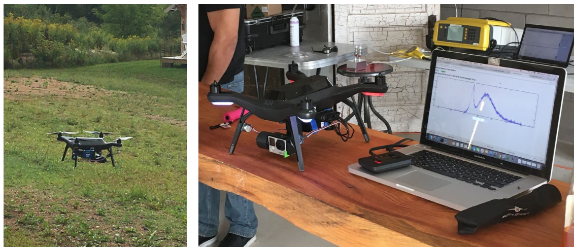
Figure 10. On the left the 3DR Solo is shown in flight carrying the Ocean Optics spectrometer. The photo on the right shows the Solo with spectrometer, a GoPro camera, and two VOC sensor chips. The laptop is displaying a real time spectrum of an LED flashlight used to align the optics.
