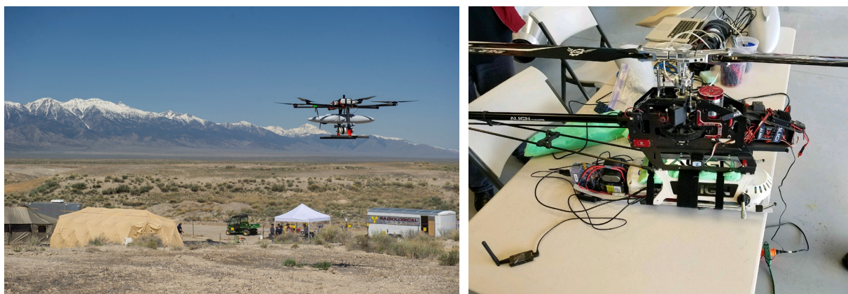
Figure 2. Left: The Virginia Tech hex-copter is carrying the Apollo detector and a 2x2 NaI(Tl) detector during an exercise at INL's RRTR. Right: The Apollo detector is strapped to a T-Rex 700 RC helicopter.
