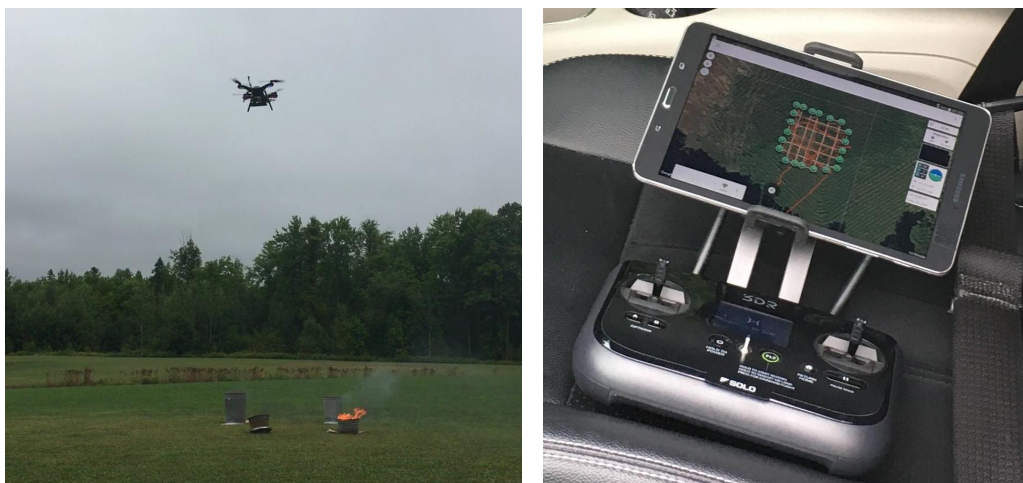
Figure 7. The 3DR Solo is flying with the chemical sensor over four garbage cans of kerosene and acetone soaked burning rags in Antigo, Wisconsin. The tablet computer attached to the 3DR controller displays the flight plan that was uploaded to the quadcopter.
