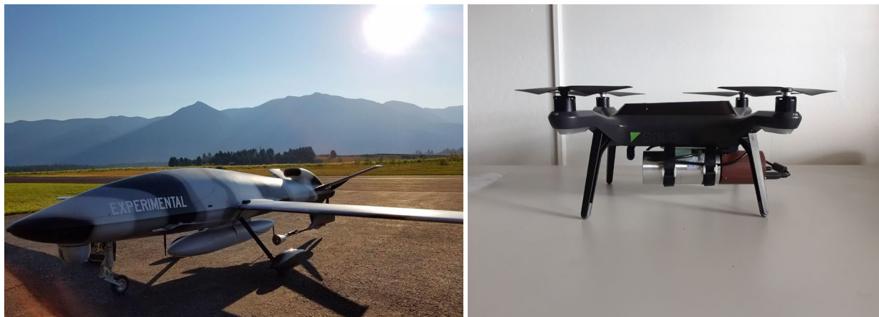
Figure 1. Left: The USI Sandstorm with the chemical detector during an exercise in Montana. Right: The 3DR Solo has a 2x2 NaI(Tl) radiation detector strapped to the expansion bay.
