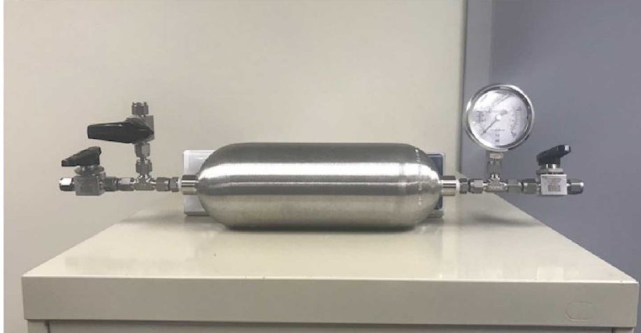
Figure 1. Sample Bottles, as Designed by Dominion Energy.
