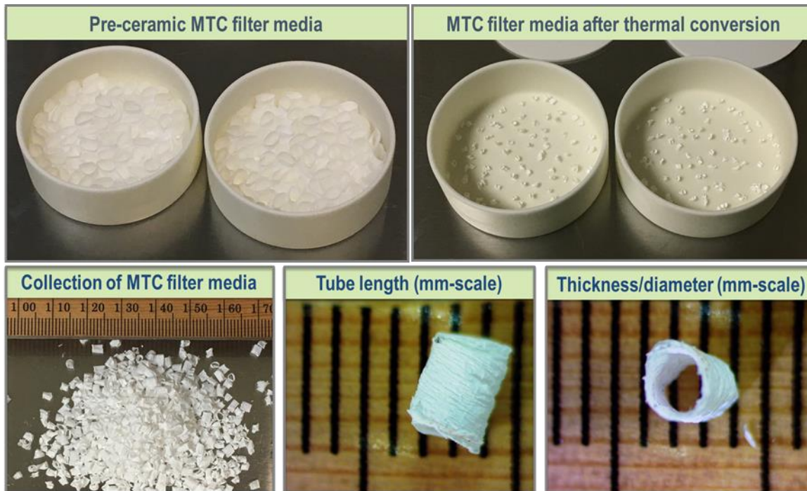
Figure 9. Images of pre-ceramic mini-tubular ceramic (MTC) filter media, before thermal treatment, and MTC filter media after thermal treatment. The MTC filter media has reasonable handling strength.
