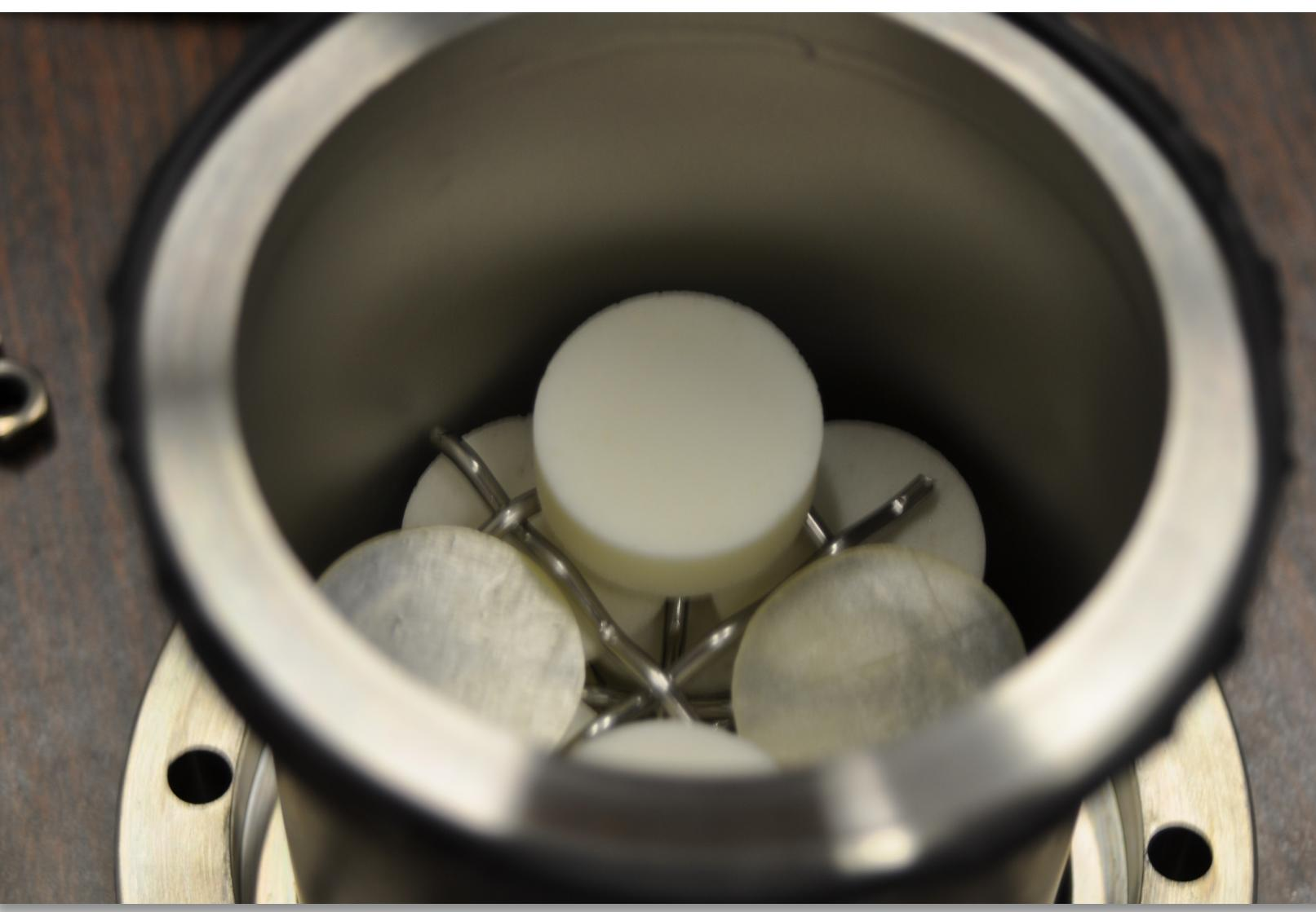
Canister with conflat flange and with stainless steel grating separating the samples
