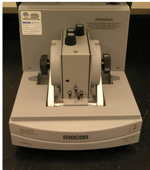
New more sensitive MOCON Ox-Tran 2/21 permeation system
