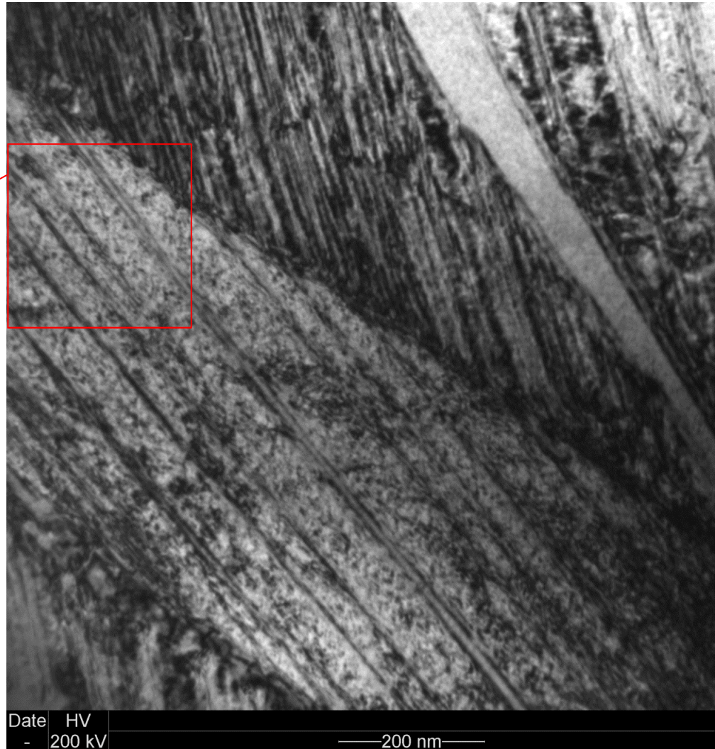
General microstructure showing martensite laths and very fine ppt. phase at room temperature
