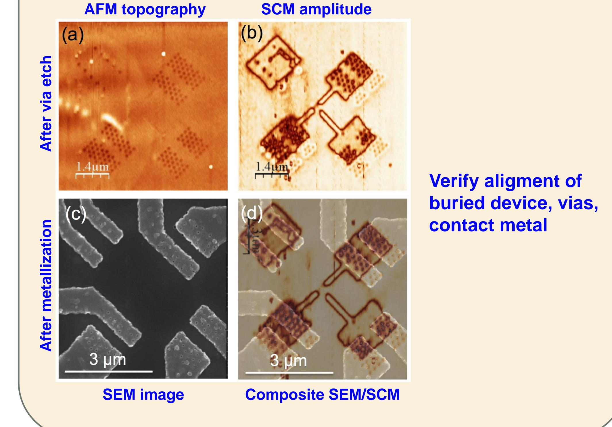
Verify alignment of buried device, vias, contact metal
