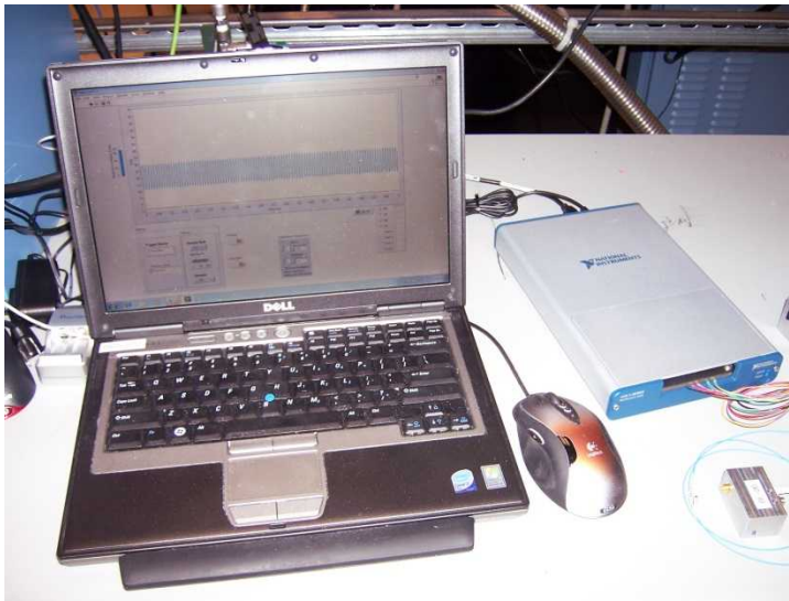
Portable data collection using laptop and digitizer
