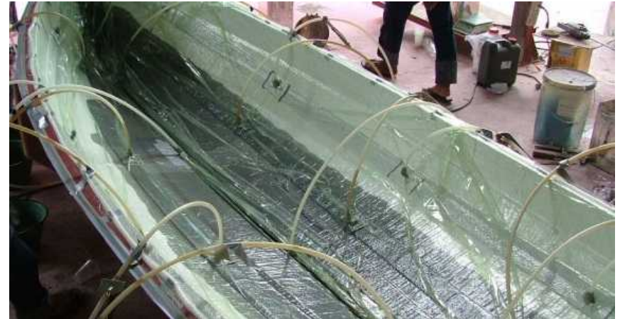
VARTM process to form the hull of a boat
